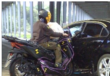
Crash test of airbag under development
